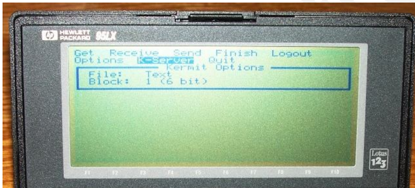
Figure 18 —Set the HP95LX in K-Server mode.
