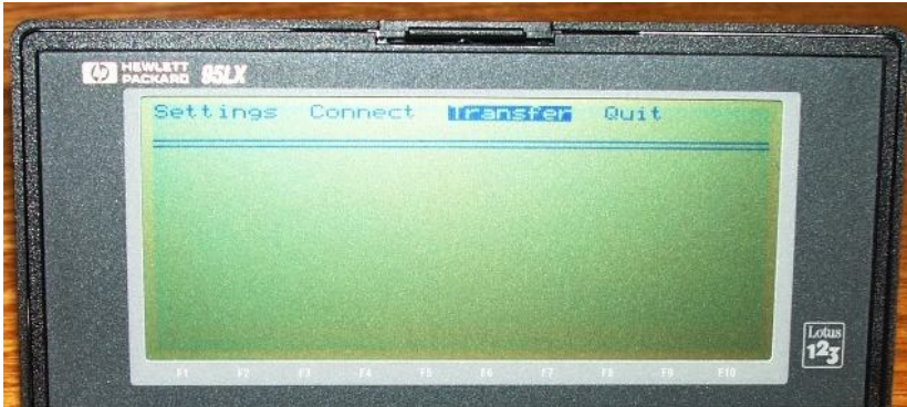
Figure 11 —Press the COMM key on the HP95XL and select the option Transfer and press ENTER.
