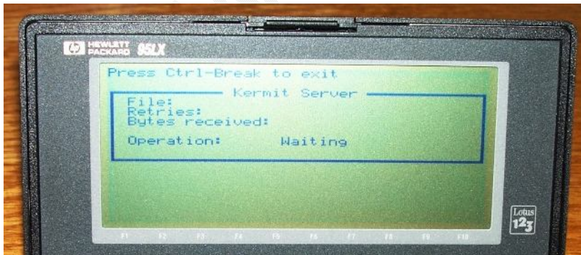
Figure 19 —The HP95LX is running K-Server (Kermit Server) and ready to receive data files.
