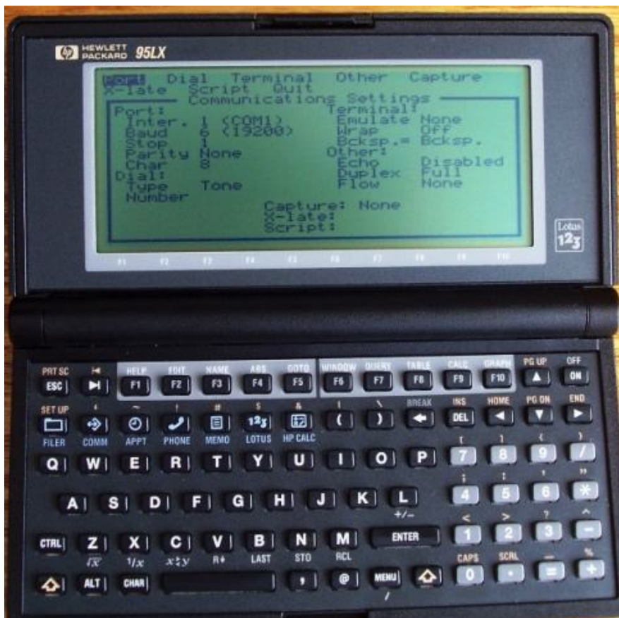
Figure 9 —After selecting the Config option, the top menu on the left image is shown. Select the Port option.
