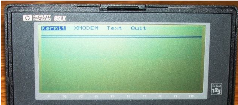
Figure 12 —Once under the Transfer screen, select the Kermit protocol and press ENTER.
