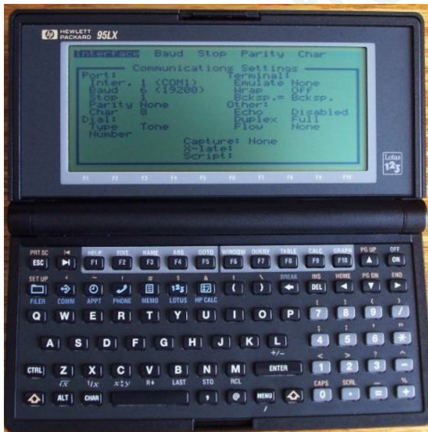
Figure 10 —Once under the Port options, the Interface, Baud, Stop, Parity and Character settings can be changed.
